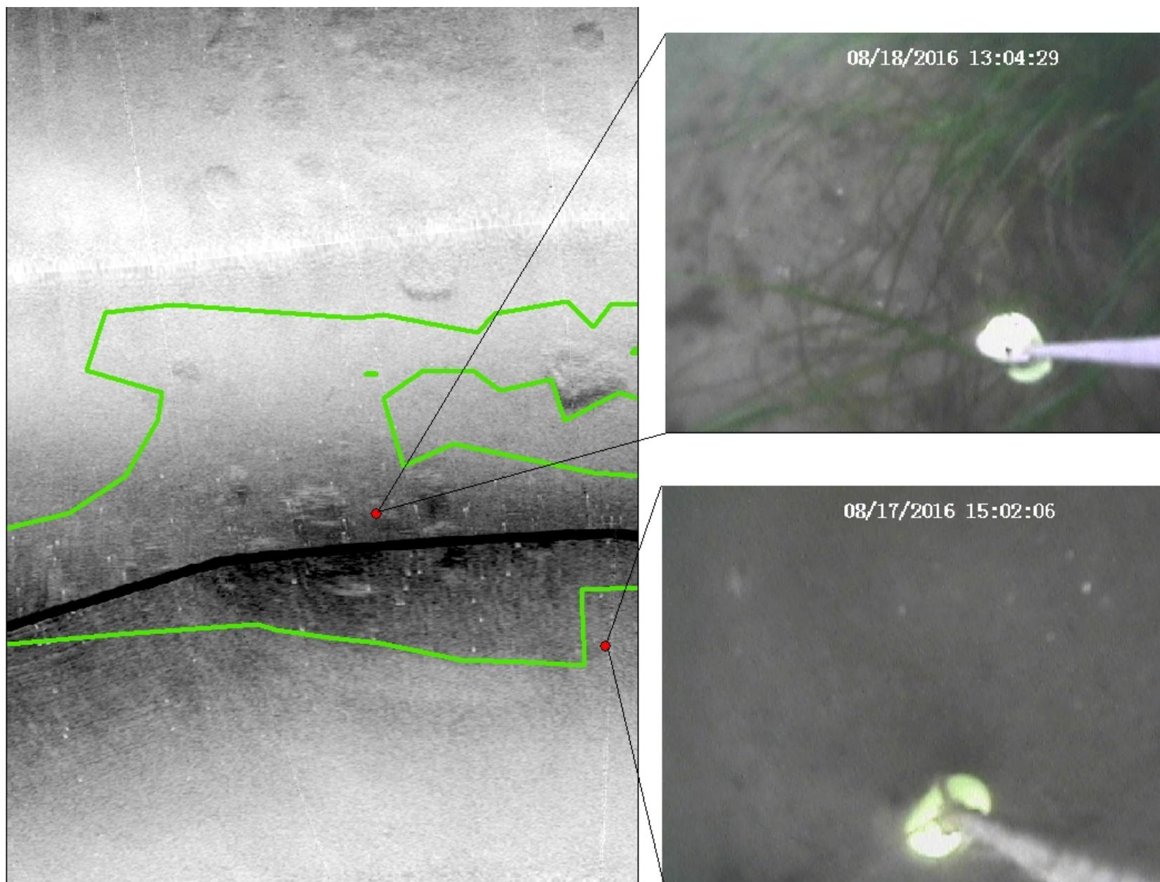
Figure 12. Locations of groundtruth points overlaid on acoustic survey imagery (left) at Woodbury Point in 2016 with corresponding groundtruth images showing an eelgrass patch (top right) and a bare sand patch (bottom right).
