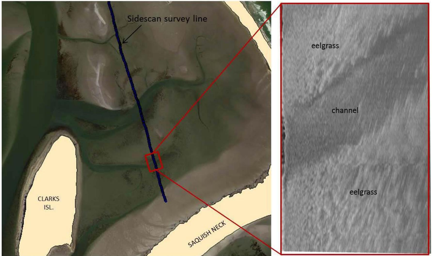
Figure 11. Example in Duxbury Bay of sidescan image output showing the signature of eelgrass versus unvegetated bottom.
