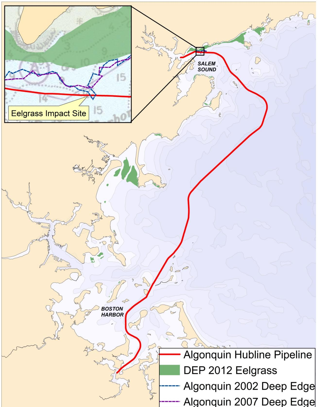
Figure 1. Location of the Algonquin Hubline Liquid Natural Gas Pipeline and the eelgrass impact site.
