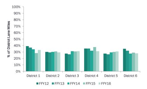
Figure 8. Pavement repair backlog (%) by Highway District
