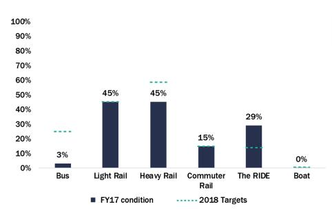
Figure 72. Percent of revenue vehicle condition at or older than ULB by line/mode
