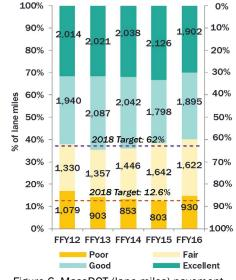
Figure 6. MassDOT (lane miles) pavement condition
