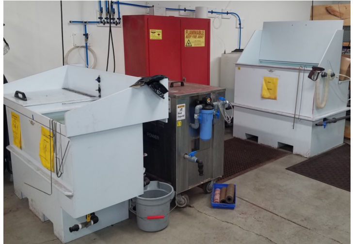
Right to Left: Benzyl Alcohol Lacquer Strip and Rinse, Ultrasonic Aqueous System, Rinse Tank
