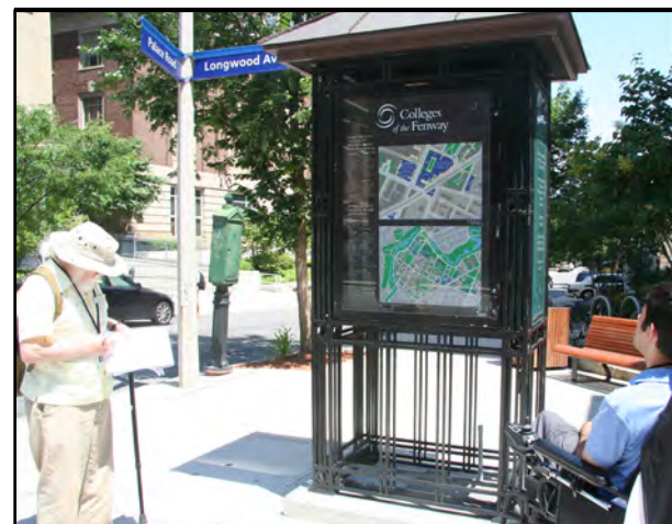
FIG. EXTERIOR- Longwood/Huntington directory difficult to read small characters are too high for a person who is seated.
