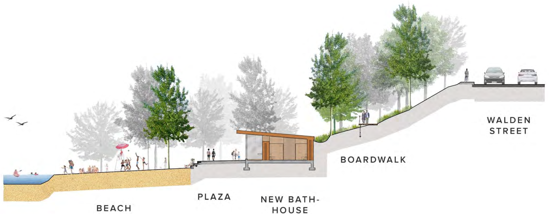
Site Section Through Bathhouse
