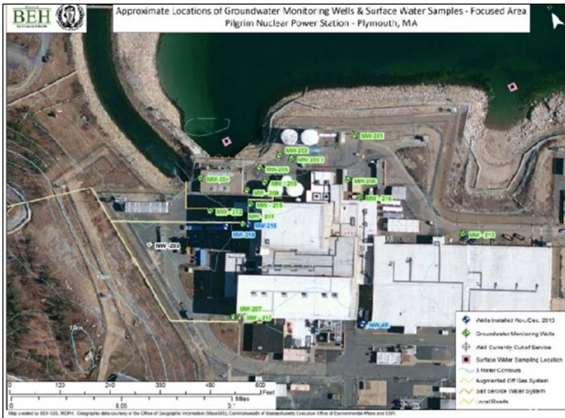
Figure 4. Approximate locations of groundwater monitoring wells around the Pilgrim facility. (Source: MassDPH)
