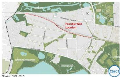
Evaluate building a flood wall at elevation 22.5 feet CCB South of the railroad track along the Alewife Quadrangle. Building a flood wall at this location can protect the Fresh Pond Reservoir, as well as the Alewife Quadrangle neighborhood.
