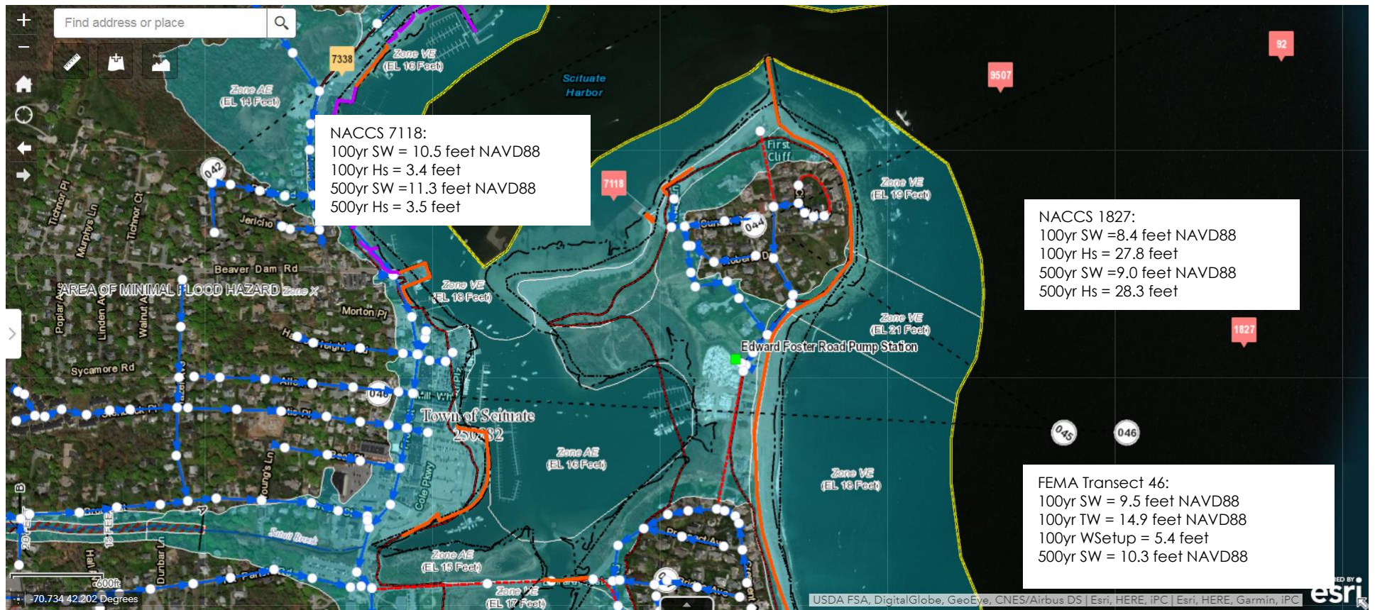
Figure 4-42: FEMA Flood Insurance Rate Map (FIRM) at Edward Foster Pump Station
