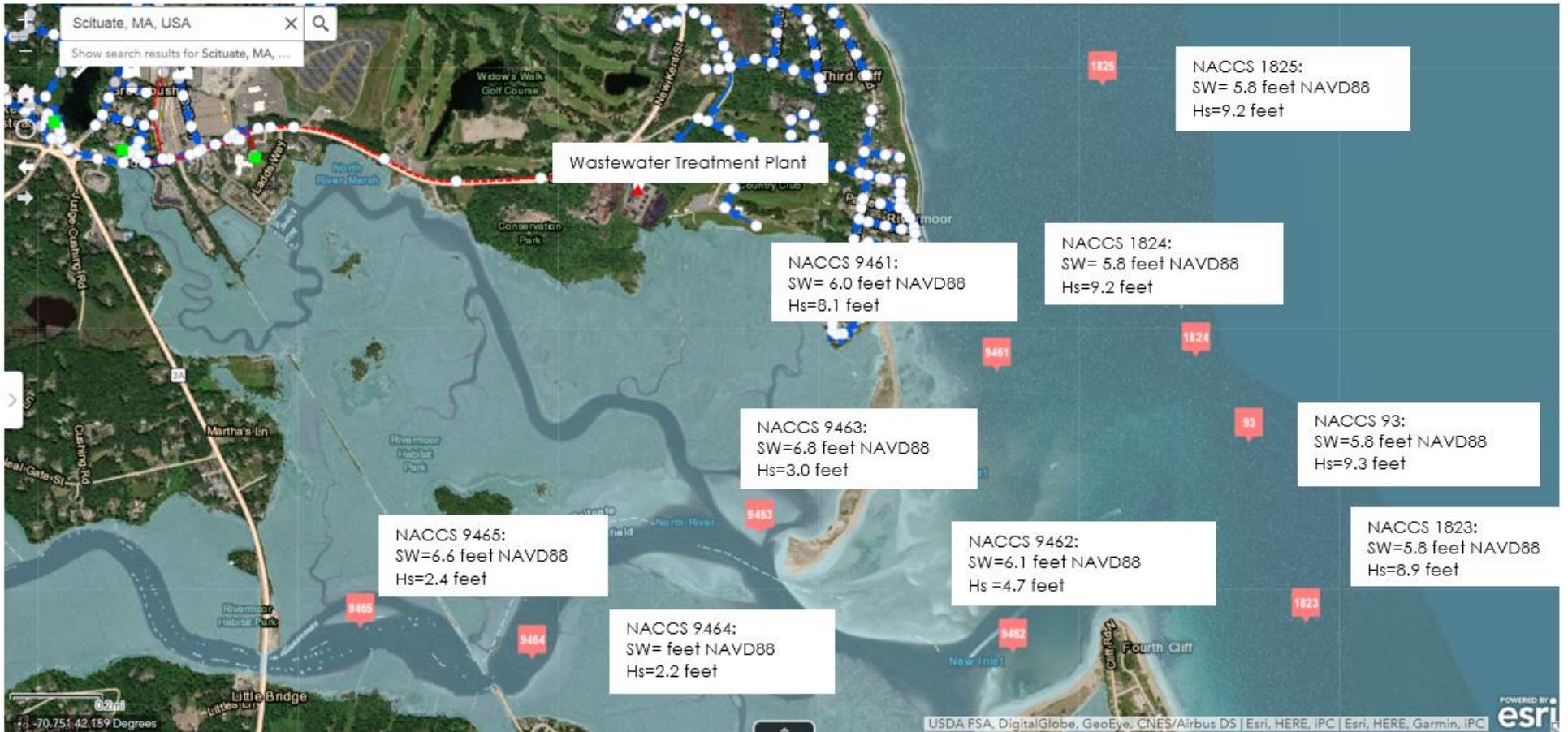
Figure 4-17: USACE NACCS 1-year Recurrence Interval Stillwater Elevations and Wave Heights (Stillwater = +/- 7 feet NAVD88)
