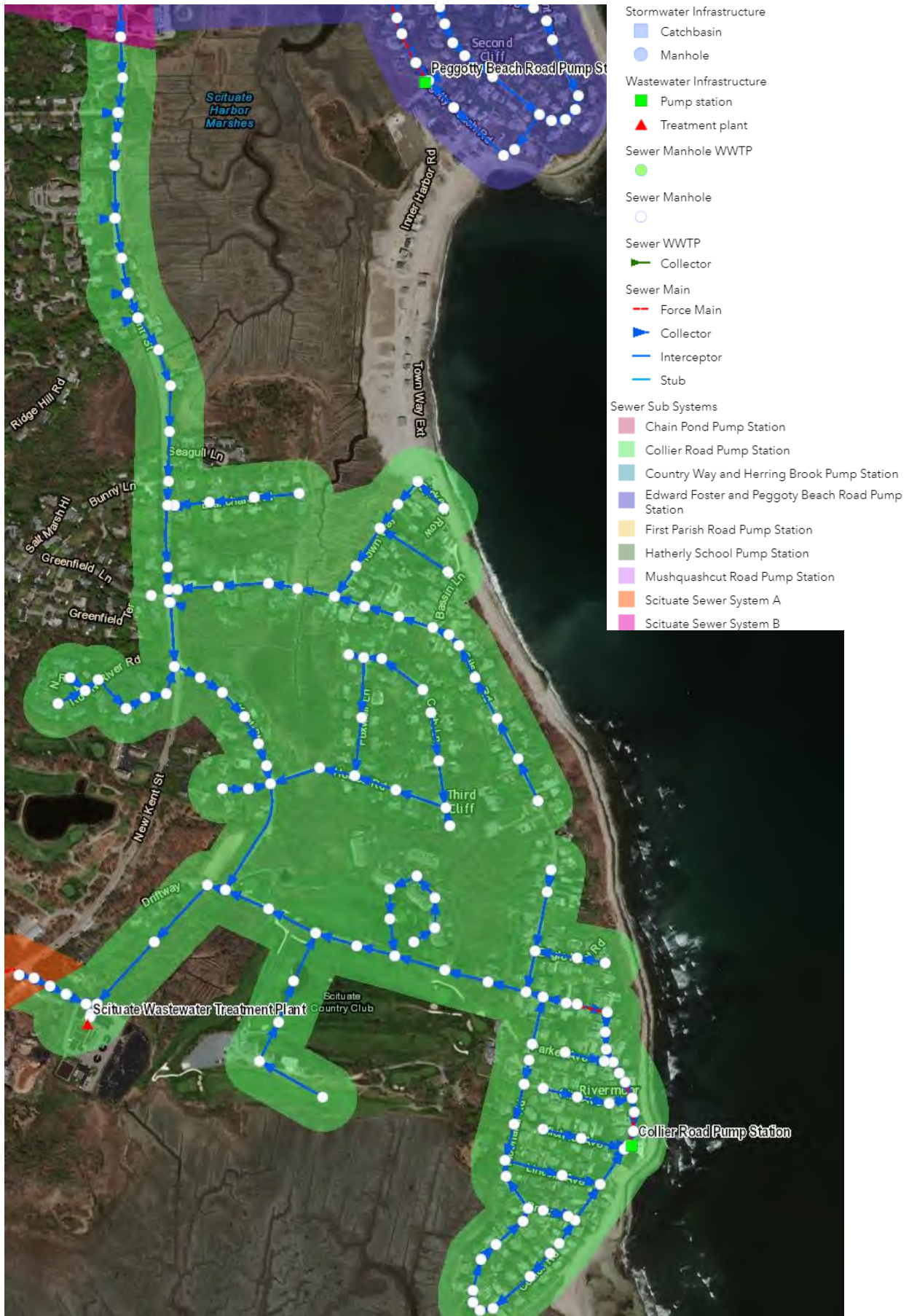
Figure 2-5: Collier Road Pup Station Sewer System
