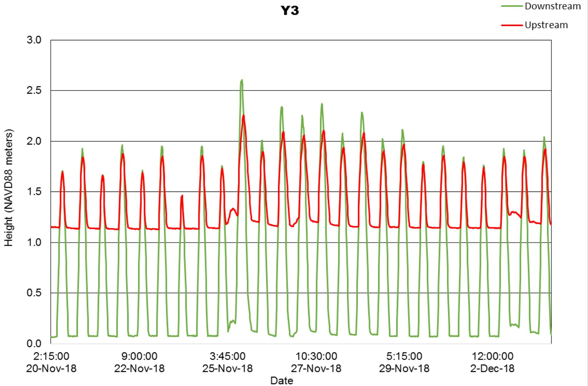
Figure 67: Hydrograph for Site Y3 from 11/20/18 to 12/3/18. Data were measured with Onset HOBO data loggers. The green (downstream) and red (upstream) lines represent the fluctuation in water height (NAVD88 meters) during the measured time period. The pulse seen on November 25 is due to a precipitation event that resulted in 3.76 centimeters (about 1.5 inches) of rainfall (NOAA 2018).
