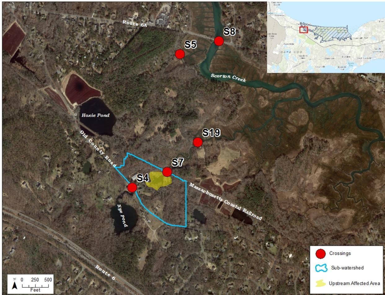
**Figure 5:** Site S7 is located at 41.7296°N 70.4294°W in Sandwich. Upstream Affected Area (as shown in the pea-green shaded area): Salt Marsh, none; Shallow Marsh, Meadow, or Fen, 2.68 acres; Shrub Swamp, none (based on the MassDEP Wetlands layer). Crossing S4 (pg. 10) is located upstream and crossings S19 (pg. 14), S5 (pg. 16), and S8 (pg. 19) are located downstream.
