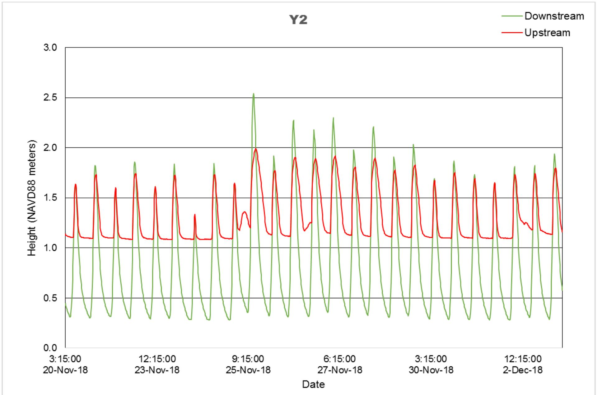
Figure 61: Hydrograph for Site Y2 from 11/20/18 to 12/3/18. Data were measured with Onset HOBO data loggers. The green (downstream) and red (upstream) lines represent the fluctuation in water height (NAVD88 meters) during the measured time period. The pulse seen on November 25 is due to a precipitation event that resulted in 3.76 centimeters (about 1.5 inches) of rainfall (NOAA 2018).
