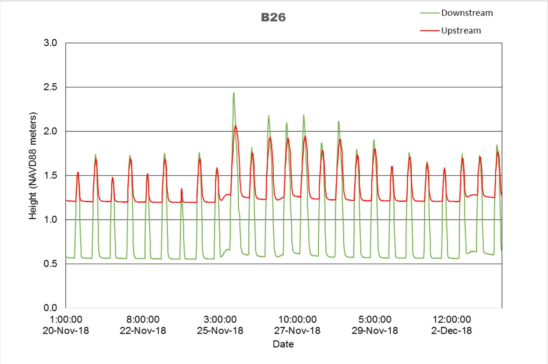
Figure 52: Hydrograph for Site B26 from 11/20/18 to 12/3/18. Data were measured with Onset HOBO data loggers. The green (downstream) and red (upstream) lines represent the fluctuation in water height (NAVD88 meters) during the measured time period. The pulse seen on November 25 is due to a precipitation event that resulted in 3.76 centimeters (about 1.5 inches) of rainfall (NOAA 2018).
