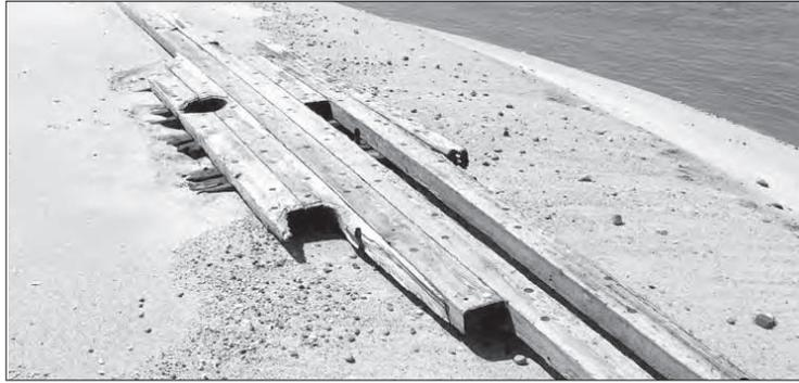
The wreckage shows hull planks, some with joints that still appear tight, over the remaining fragments of ribs. COURTESY MIKE RYDER
