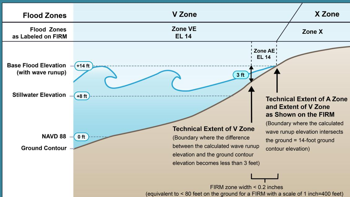
Figure 1.16. Cross-sectional diagram of flood zones on a steep embankment with runup. Here, an A Zone is shown in the profile, but would not be mapped on the FIRM because the zone is less than 0.2 inches in width on the FIRM—thereby not meeting the minimum zone width for mapping at the scale used for FIRMs. Where A Zones such as these are not mapped, the V Zone will extend to the designated ground elevation that corresponds to the V Zone BFE on the FIRM.
