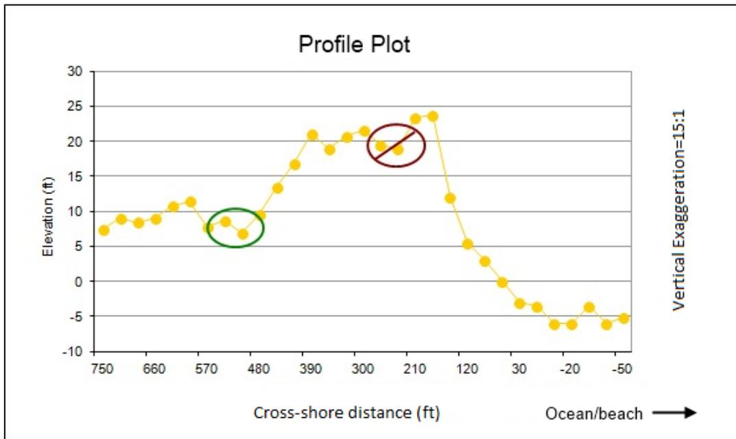
To determine the maximum possible extent of the primary dune, the applicant will need to determine the seaward point and then the landward point as follows:
