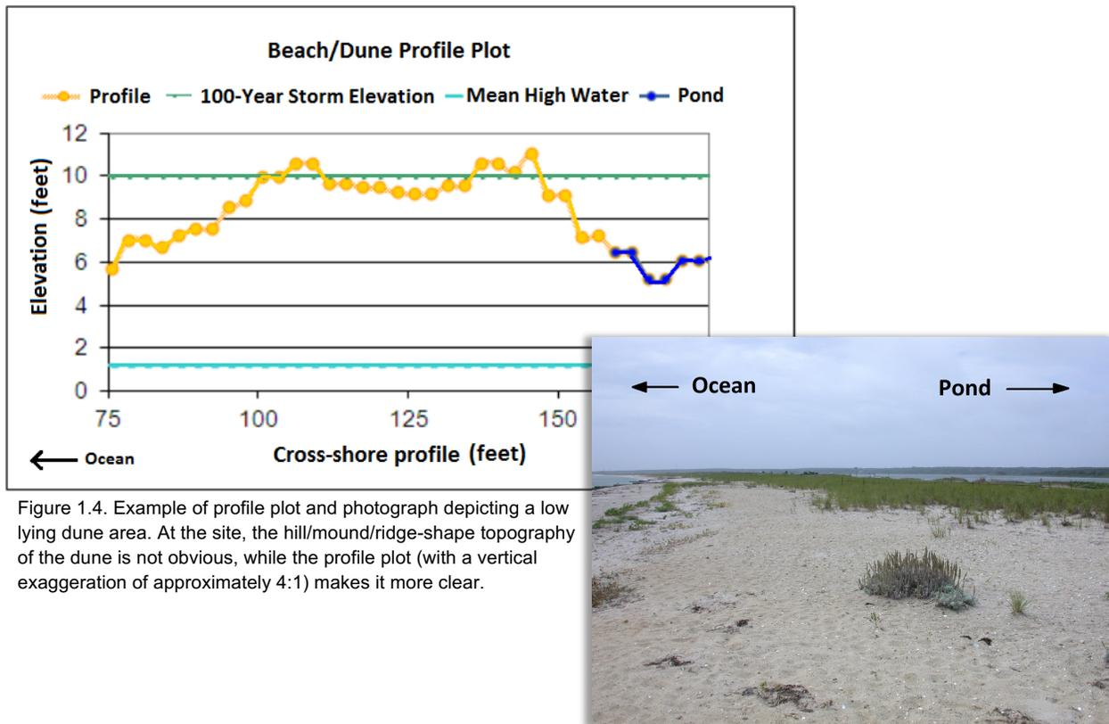
Figure 1.4. Example of profile plot and photograph depicting a low lying dune area. At the site, the hill/mound/ridge-shape topography of the dune is not obvious, while the profile plot (with a vertical exaggeration of approximately 4:1) makes it more clear.
