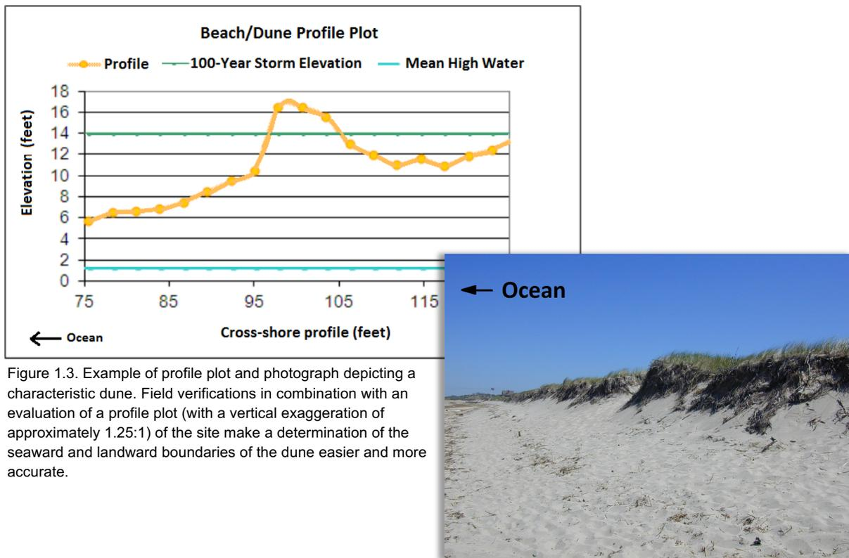
Figure 1.3. Example of profile plot and photograph depicting a characteristic dune. Field verifications in combination with an evaluation of a profile plot (with a vertical exaggeration of approximately 1.25:1) of the site make a determination of the seaward and landward boundaries of the dune easier and more accurate.
