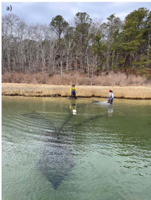
Figure 2. Images of fyke nets deployed in Waquoit Bay. View A (left) looks shoreward from the codend of the trap towards the wings and leadline anchored to the shoreline while. View B (right) looks seaward toward the wings and codend.
