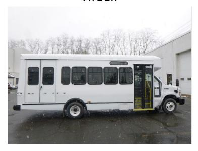
Raised-roof "body-on-chassis cutaway," dual rear wheel, with wheelchair lift. The vehicle seats up to 16 ambulatory passengers and two wheelchair positions, 14 ambulatory passengers and three wheelchair positions, or 10 ambulatory passengers and four wheelchair positions.
