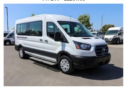
Medium-roof van, single rear wheel, with rear wheelchair lift. The vehicle seats four ambulatory passengers and two wheelchair positions. Comes with a wall charger, 120V/240V mobile power cord, and an on-board charger (10.5 kW out/11.3 kW in).
