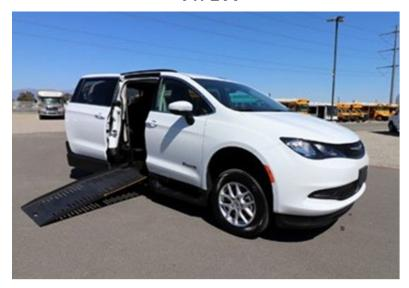
Minivan style vehicle with one or two wheelchair positions and electronic accessibility ramp. The vehicle seats six ambulatory passengers, four ambulatory passengers and one wheelchair position, or three ambulatory passengers and two wheelchair positions.
