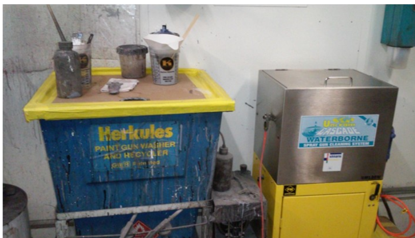
Old paint gun washers. Herkules solvent unit was replaced with another Uniram as on the right
