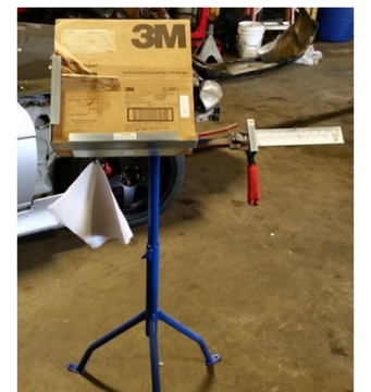
Non-lead wheel weight roll and cutting system
