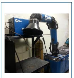
This portable fume extractor features an adjustable arm that pulls welding fumes away from the welder's personal breathing zone.
