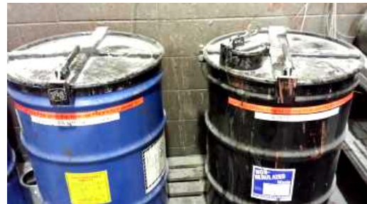
Waste Drums with One-Handed Covers
