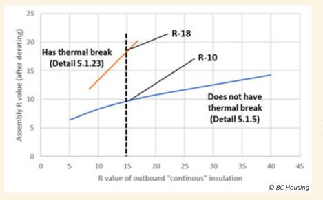
This illustration shows the derated, overall assembly performance (y-axis) as a function of the R-value of outboard continuous insulation (x-axis).
