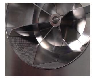
Figure 3 – Impeller and milling screen
