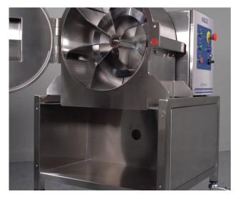
Figure 4 – Impeller and collection area, bin removed
