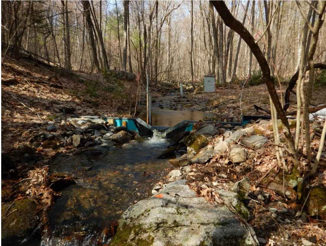
A. Weir that was installed to monitor stream flow.
