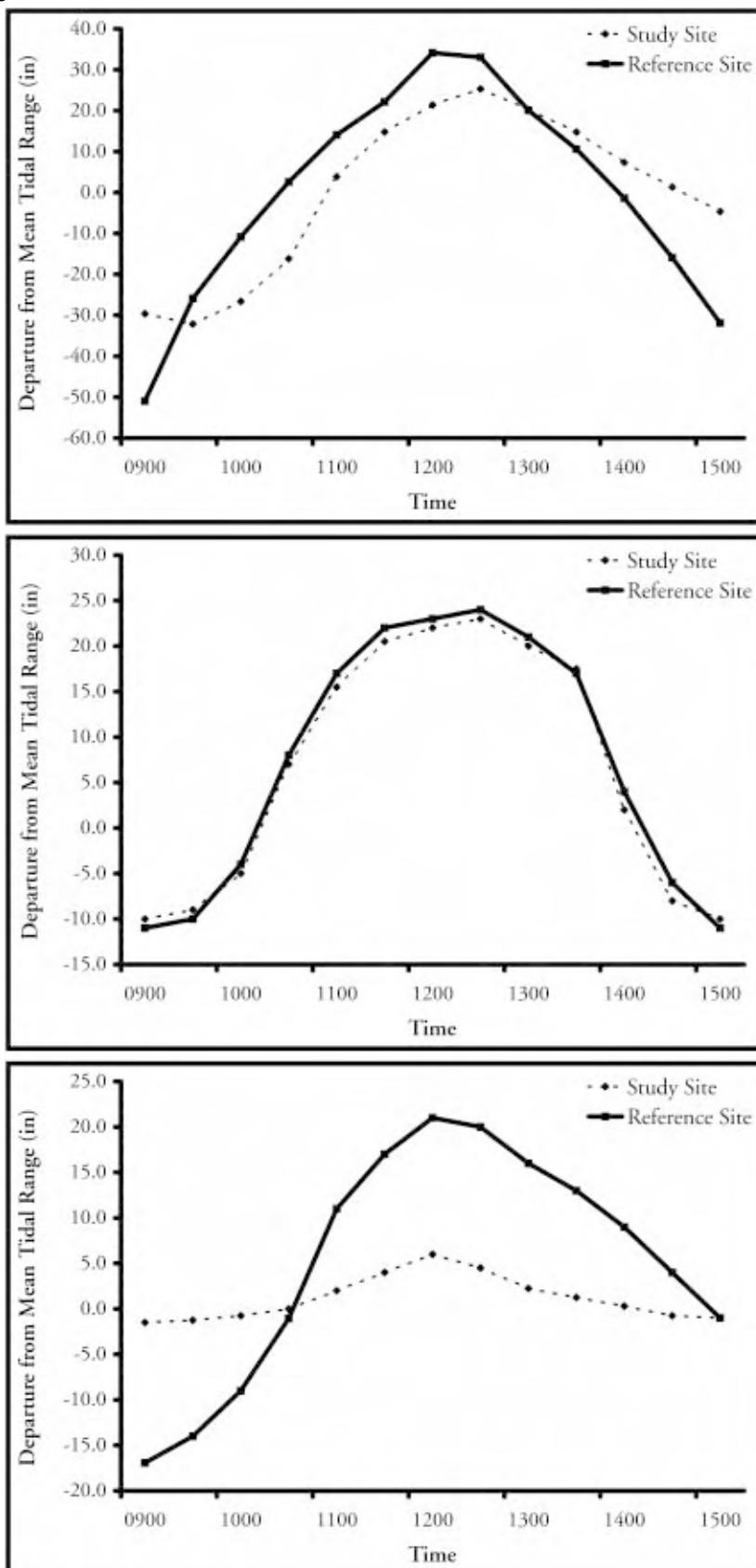
C. Tidal graph showing a severe tidal restriction caused by an insufficiently sized or collapsed culvert. The tidal peak occurs at the same time in the study site and reference site, but the change in tidal height is significantly less at the study site, indicating that water is prevented from flowing freely from one side of the marsh to the other.
