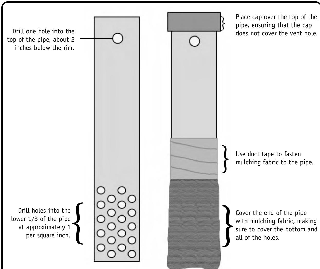
**FIGURE 1. GROUNDWATER WELL ASSEMBLY** See text for details.
