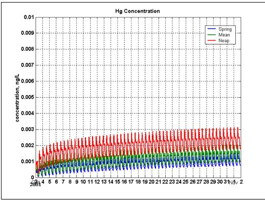
Figure 7-b. Time history of mercury concentration at the LH-CAD site for different tidal conditions. The simulation is performed with a continuous release.
