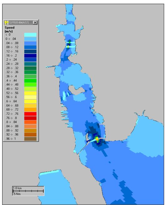
Figure 4. The modeled speed field at the ebb tide during spring tidal condition.
