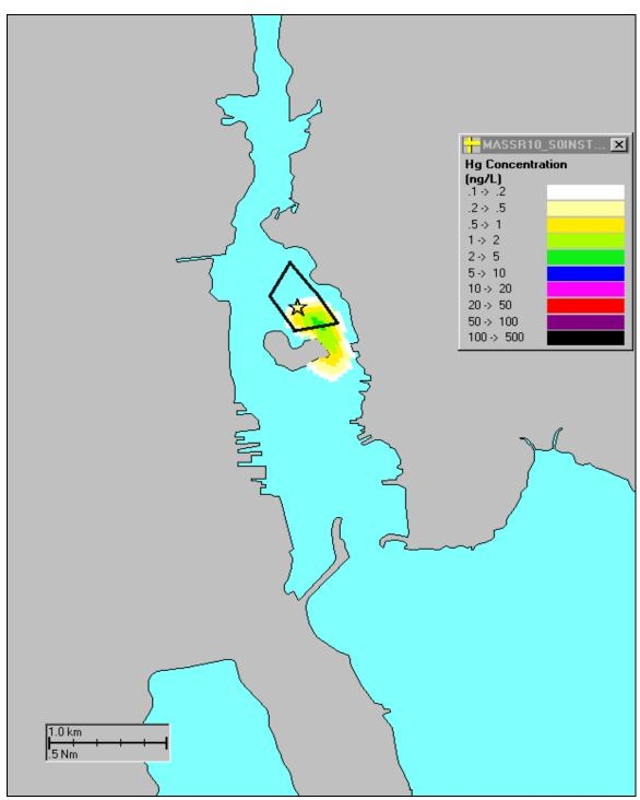
Figure 5-a. Modeled mercury (Hg) concentration (ng/L =  $0.001 \mu$ g/L) field 6 hours after a 3000 yd<sup>3</sup> instantaneous release: A star represents the release site, located at the Popes Island North CAD site (polygon).
