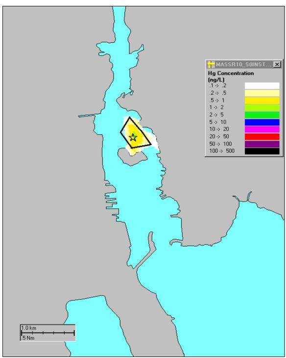
Figure 5-b. Modeled mercury (Hg) concentration ( $ng/L = 0.001 \ \mu g/L$ ) field 12 hours after a 3000 yd<sup>3</sup> instantaneous release: A star represents the release site, located at the Popes Island North CAD site (polygon).
