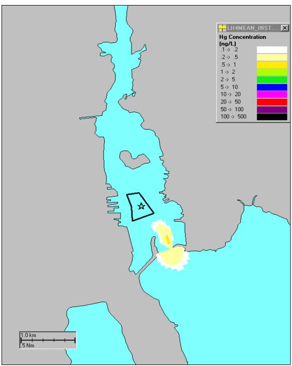
Figure 6-a. Modeled mercury (Hg) concentration ( $ng/L = 0.001 \ \mu g/L$ ) field 6 hours after a 3000 yd<sup>3</sup> instantaneous release: A star represents the release site, located at the federal navigation channel inner CAD site (polygon).
