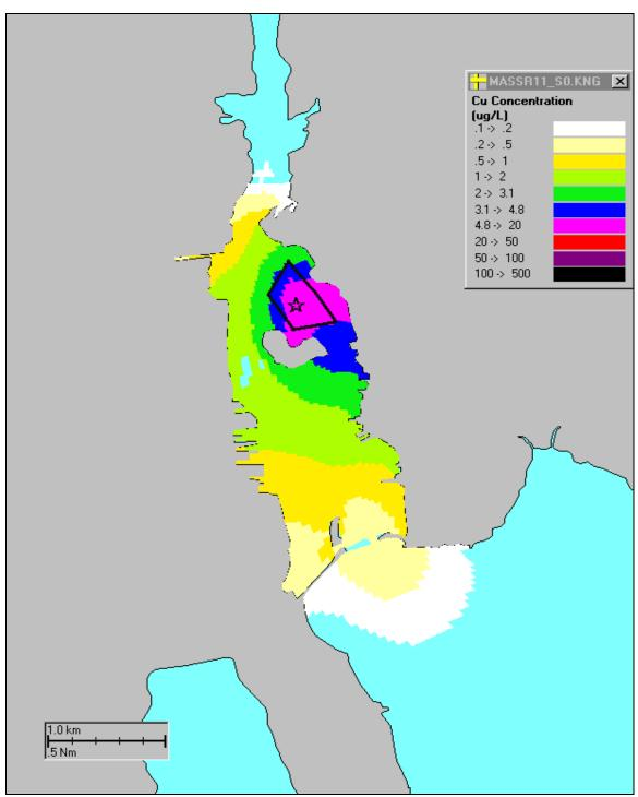
Figure 9-b. Modeled copper (Cu) concentration ( $\mu$ g/L) field during flood at simulationday 29 for a continuous release. This simulation is done during the Neap tide. A star represents the release site, located at the PI-CAD site (polygon).
