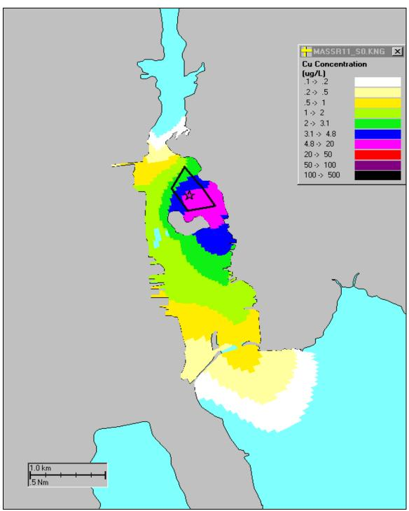
Figure 9-a. Modeled copper (Cu) concentration ( $\mu$ g/L) field during ebb at simulation-day 29 for a continuous release. This simulation is done during the Neap tide. A star represents the release site, located at the PI-CAD site (polygon).
