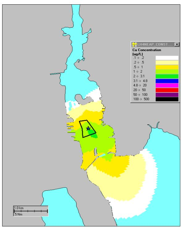
Figure 10-a. Modeled copper (Cu) concentration ( $\mu$ g/L) field during ebb at simulationday 29 for a continuous release. This simulation is done during the Neap tide. A star represents the release site, located at the LH-CAD site (polygon).
