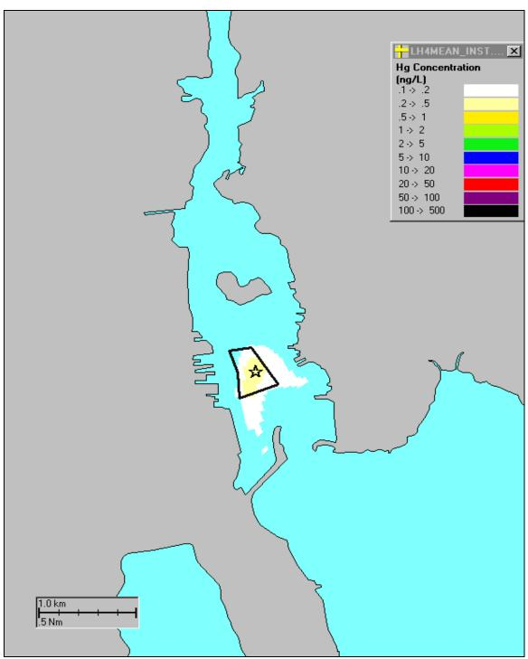
Figure 6-b. Modeled mercury (Hg) concentration ( $ng/L = 0.001 \ \mu g/L$ ) field 12 hours after a 3000 yd<sup>3</sup> instantaneous release: A star represents the release site, located at the federal navigation channel inner CAD site (polygon).
