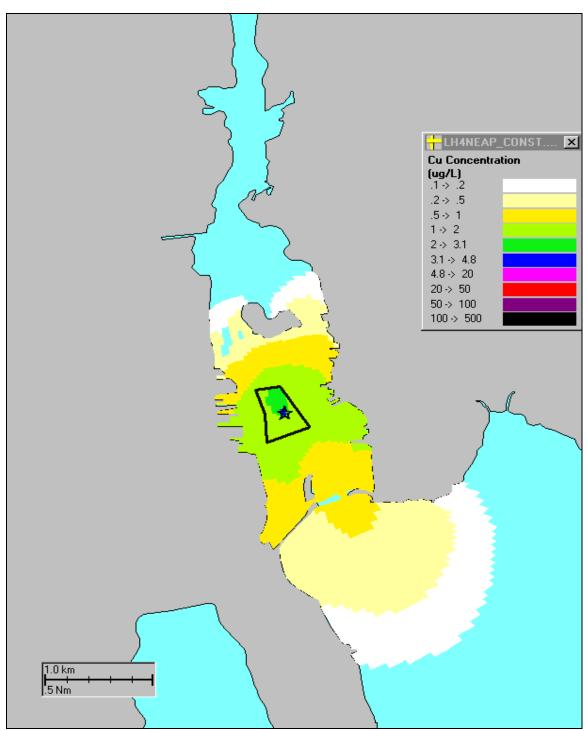
Figure 10-b. Modeled copper (Cu) concentration ( $\mu$ g/L) field during flood at simulationday 29 for a continuous release. This simulation is done during the Neap tide. A star represents the release site, located at the LH-CAD site (polygon).
