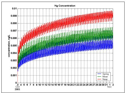
Figure 7-a. Time history of mercury concentration at the PI-CAD site for different tidal conditions. The simulation is performed with a continuous release.
