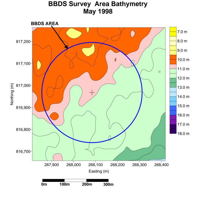
**Figure 3-3.** Bathymetric results from the BBDS Survey Area (NAD 83), contour interval = 0.2 m.
