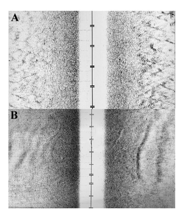
**Figure 2-3.** Examples of bottom textures from side-scan data showing (A) ambient bottom and (B) sand waves.
