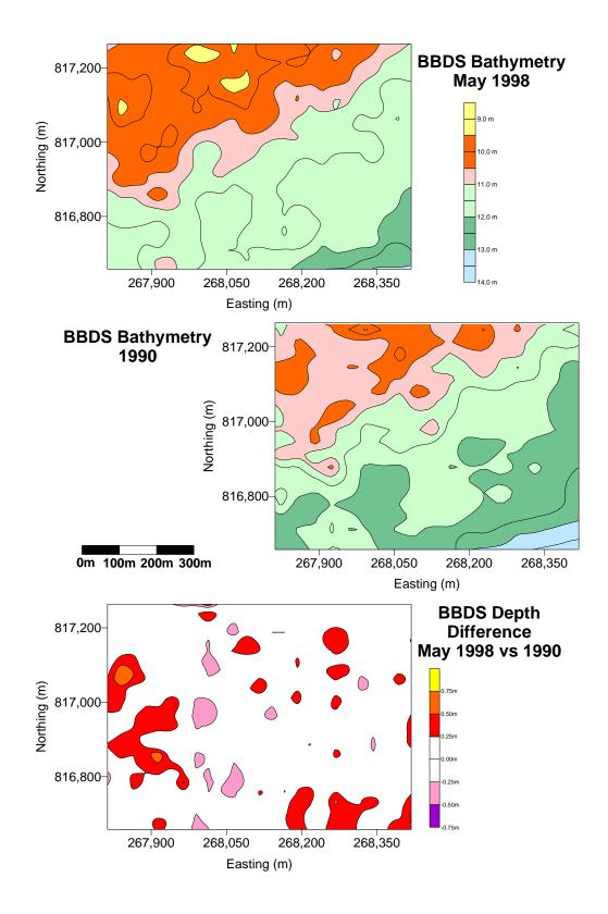
**Figure 3-4.** Depth difference results (bottom) from the 1998 (top) and 1990 (middle) bathymetric surveys.
