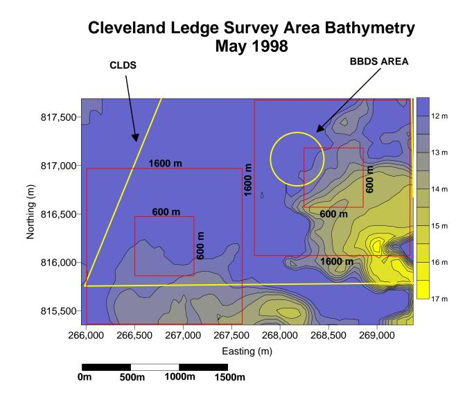
**Figure 4-1.** Bathymetry of the Cleveland Ledge Survey Area highlighting water depths of greater than 12 m.
