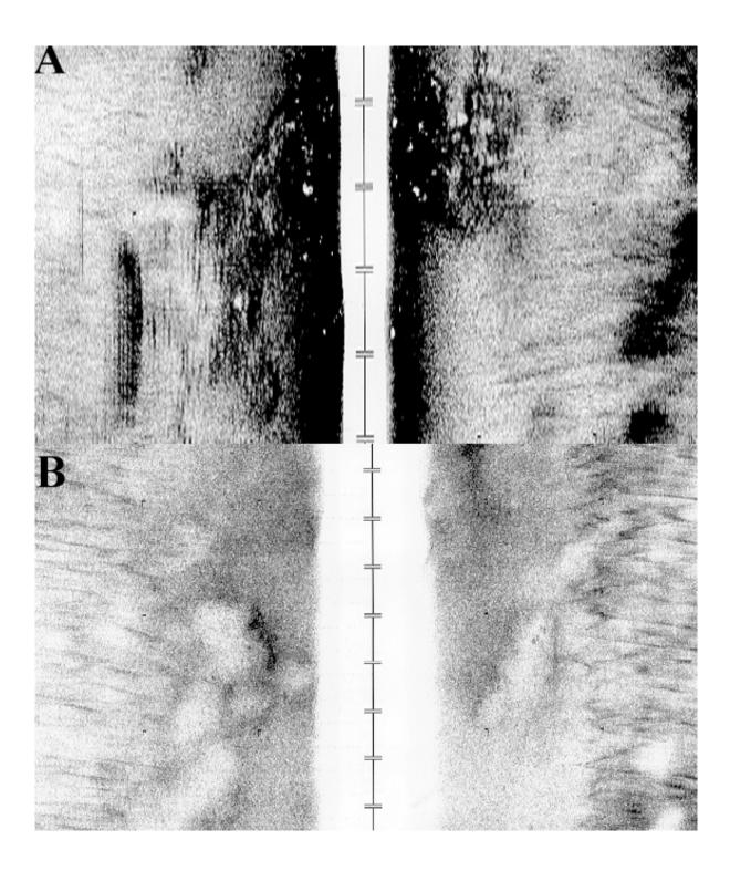
**Figure 2-1.** Examples of the acoustic appearance of dredged material, including (A) rubbled texture and (B) cratered texture.
