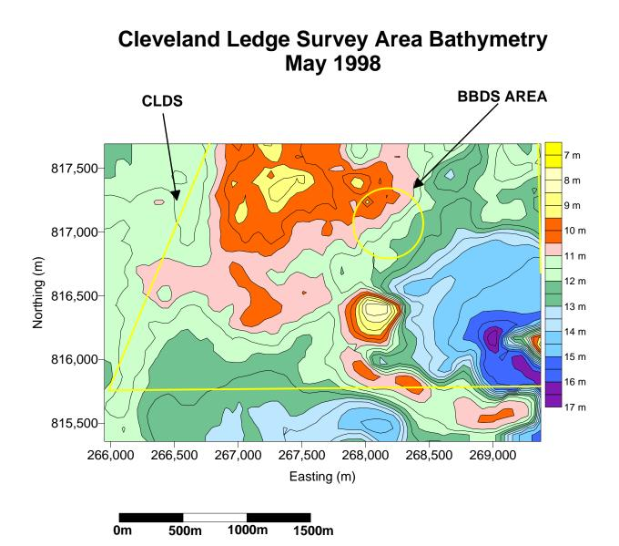
**Figure 3-1.** Bathymetric results from the Cleveland Ledge Survey Area (NAD 83), contour interval = 0.5 m.
