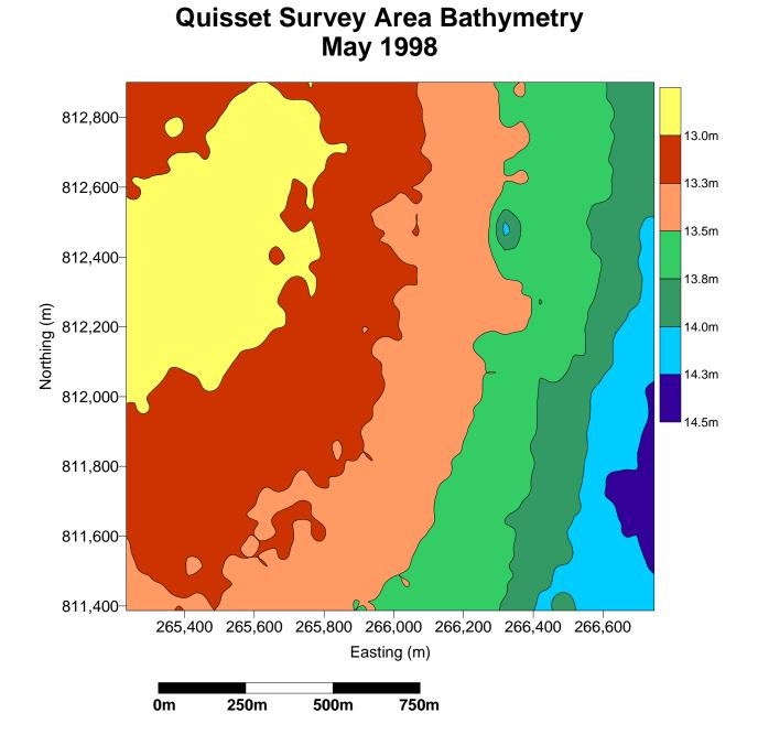
**Figure 3-5.** Bathymetric results from the Quisset Survey Area (NAD 83), contour interval = 0.2 m.
