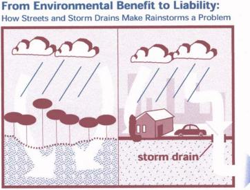
An urban environment changes the natural water cycle. Rain that would seep into groundwater on undeveloped land instead rushes over asphalt into storm drains and away to rivers and the ocean.
