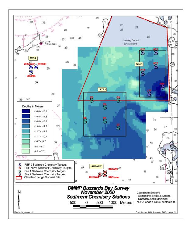
**Figure 2-1.** Map showing the location of sediment chemistry sampling stations at candidate disposal Sites 1 and 2 and reference areas Ref-New and Ref-2. Color bathymetry results underlying Sites 1 and 2 are in meters, from SAIC surveys conducted in May 1998 and October 2000. Depth values on the underlying NOAA chart are in feet.
