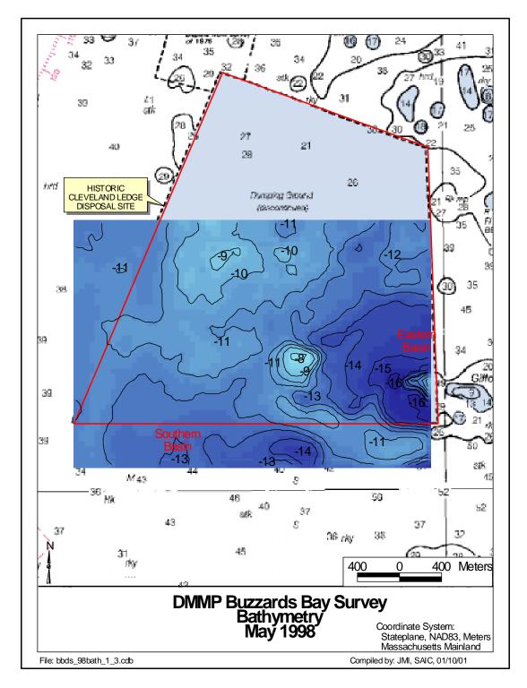
**Figure 1-3.** Results of the high-resolution bathymetric survey conducted across the southern half of the Cleveland Ledge Disposal Site in May 1998, superimposed on NOAA Nautical Chart 13229. Depths from the bathymetric survey are in meters; nautical chart depth soundings are in feet.
