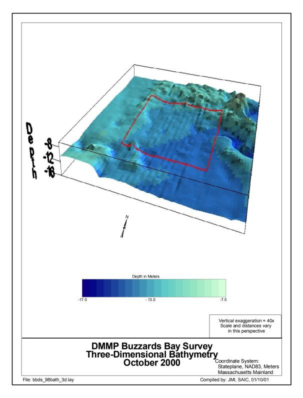
**Figure 3-2.** Three-dimensional representation of the October 2000 bathymetric survey results at candidate Site 1 (note: vertical exaggeration of 40X causes scale and distances to be distorted in this perspective).
