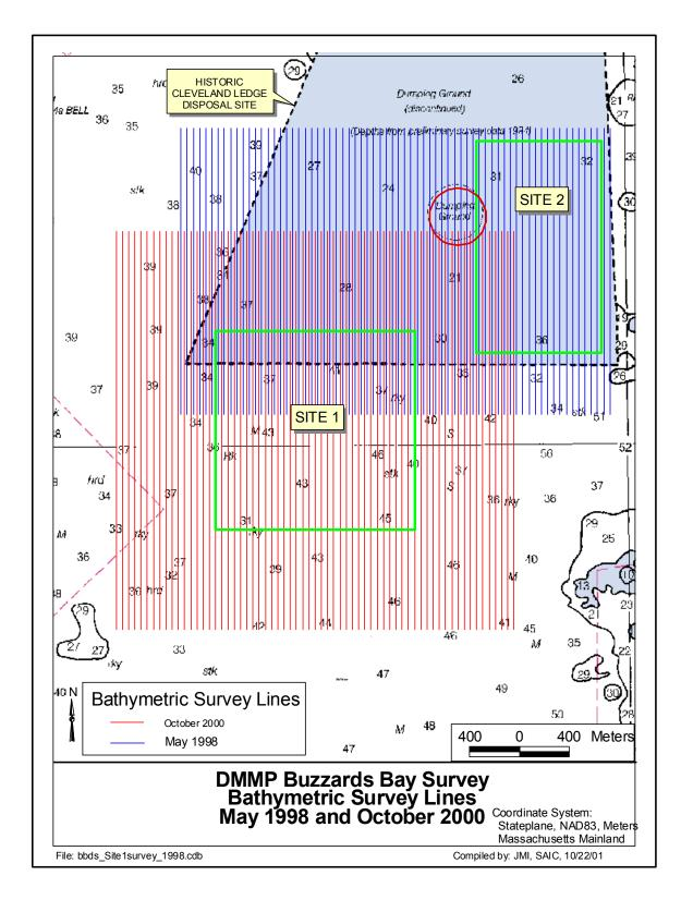
**Figure 2-1.** Map showing bathymetric survey lines occupied around Site 1 in October 2000 (red) and the survey lines from the May 1998 bathymetric survey (blue).
