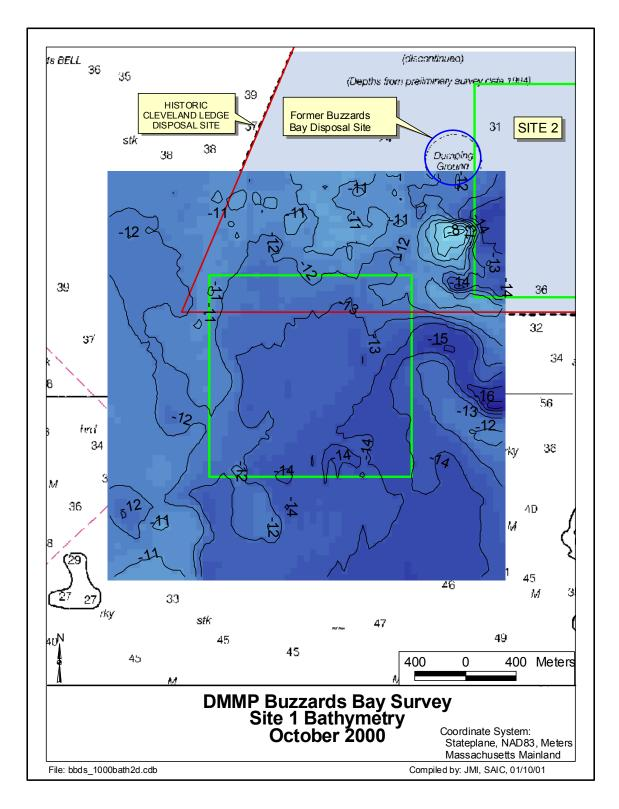
**Figure 3-1.** Map showing depth contours (in meters) in and around candidate Site 1, superimposed on NOAA Nautical Chart 13229. Depth soundings on the underlying NOAA chart are in feet.
