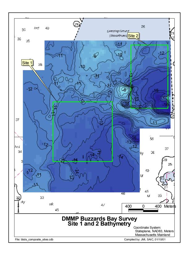
**Figure 3-5.** Two-dimensional contour map showing bottom topography in and around candidate disposal Sites 1 and 2 based on the combined results of the May 1998 and October 2000 bathymetric surveys.
