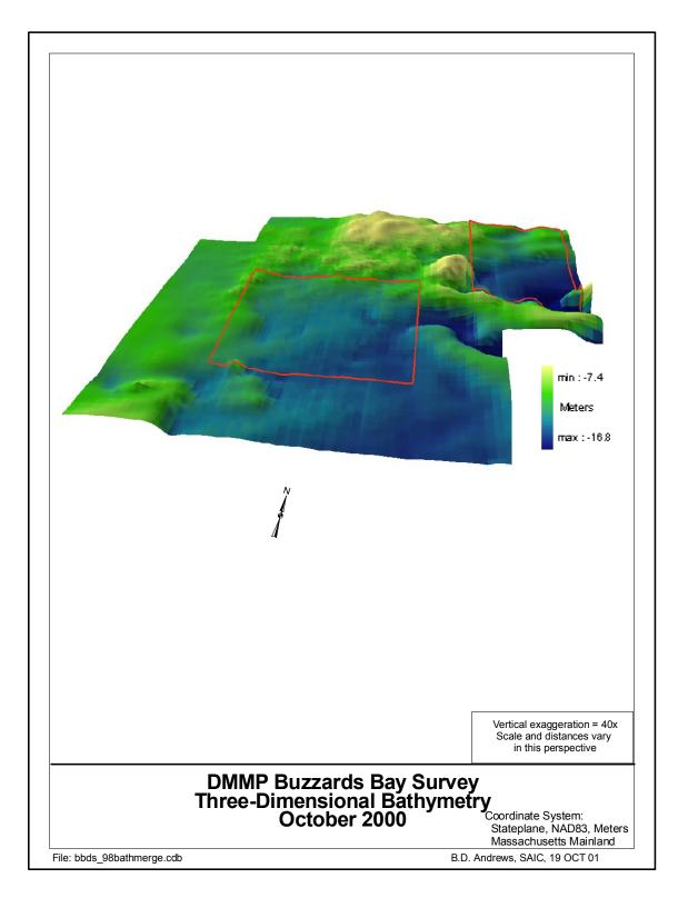
Figure 3-6. Three-dimensional map showing bottom topography in and around candidate disposal Sites 1 and 2 based on the combined results of the May 1998 and October 2000 bathymetric surveys (vertical exaggeration = 40x).
