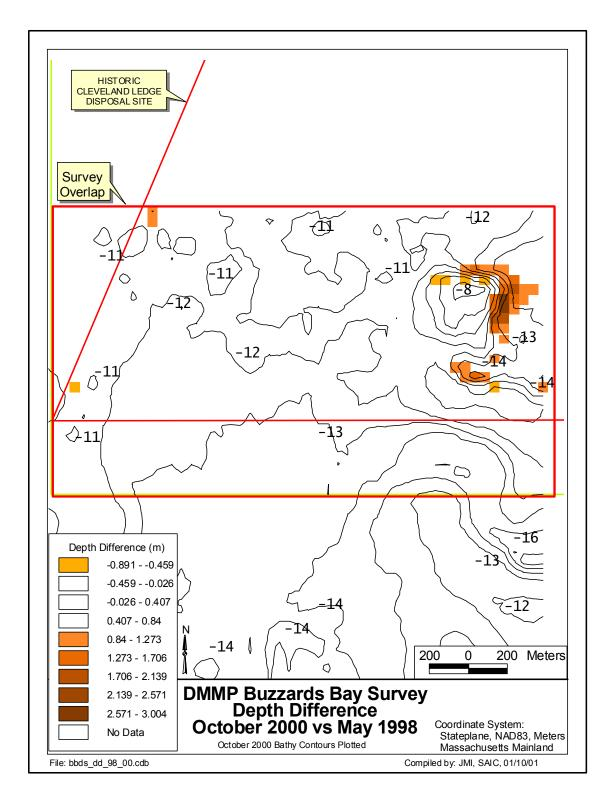
**Figure 3-4.** Map showing the results of the depth difference comparison between the October 2000 and May 1998 bathymetric surveys. The depth difference results (in meters) are superimposed on the bathymetric contours from the October 2000 survey.
