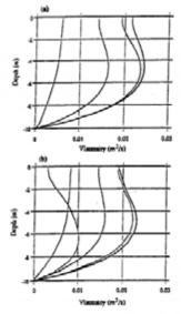
FIG. 8. Comparison of (a) Model Predicted Vertical Structure of Viscosity with (b) Numerical Simulations of Davies and Jones (1990) for One-Dimensional Turbulence Model Test Driven by  $M_{\rm p}$ Tide with imposed Pressure Gradient of 0.14 N/m<sup>2</sup>; No-Silp Bottom Boundary Condition;  $\gamma = 0.4$ ;  $\Delta t = 558.9$  s; and 40 Vertical Levels
