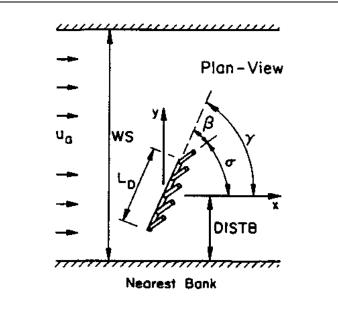
Figure 4-1b. Section view of diffuser with input parameters (reproduced from Jirka et al., 1996).
