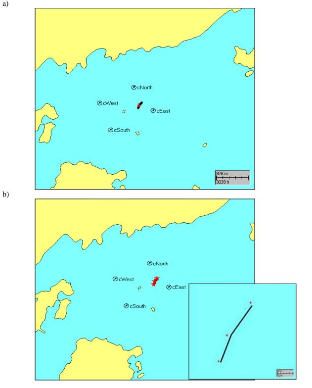
Figure 5-7. Load location (star): a) single source, b) distributed source (three cells), with insert of the detail around the outfall. a)
