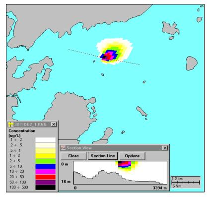
Figure 5-13. Simulated TRC concentration distribution at maximum flood (a) and maximum ebb (b) for scenario 2. Inserted vertical section view is along the dashed line in the east-west direction. (a)
