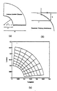
FIG. 4. Three-Dimensional Tidally Driven Model Test for: (a) Geometry; (b) Bathymetry; and (c) Grid Configuration ( $r_1 = 5,950$  m;  $r_2 = 31,250$  m; h = 5 ( $r/r_1$ )<sup>2</sup>
