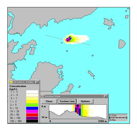
Table 5-6. Horizontal areal coverage of TRC (greater than  $0.1 \,\mu\text{g/L}$ ) and maximum TRC value during maximum flood and maximum ebb currents.
