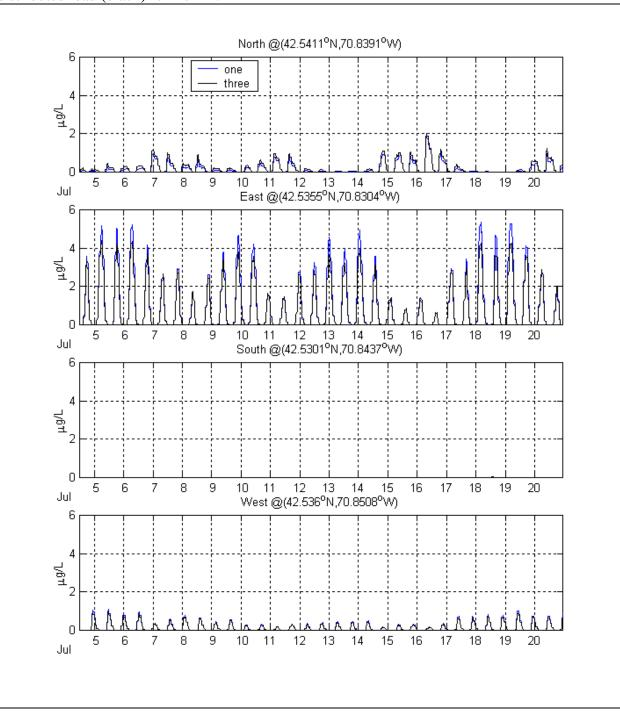
Figure 5-9. Comparison of predicted TRC concentration with single load (blue) and distributed load (black) for Run#1.
