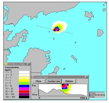
Figure 5-14. Simulated TRC concentration distribution at maximum flood (a) and maximum ebb (b) for scenario 3. Inserted vertical section view is along the dashed line in the east-west direction. (a)
