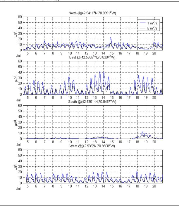
Figure 5-11. Time series of TRC concentration in the near field for different dispersion coefficients (Run#2 and Run#6).
