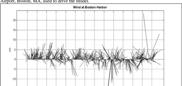
Figure 4-4. Time series of hourly wind vectors (meteorological convention) from Logan Airport, Boston, MA, used to drive the model.
