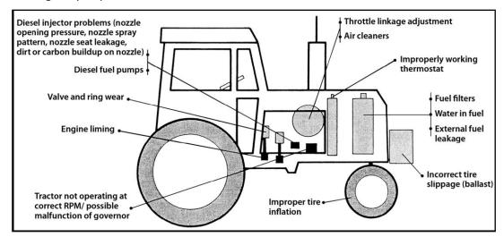
Figure 1. Factors reducing fuel efficiency on a diesel tractor (<u>http://attra.ncat.org/attra-pub/PDF/consfuelfarm.pdf</u>)
