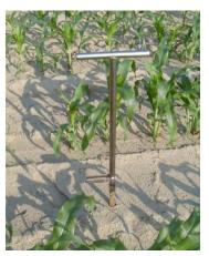
Figure 1. Sample 10 to 12 inches from the surface of the ground.
