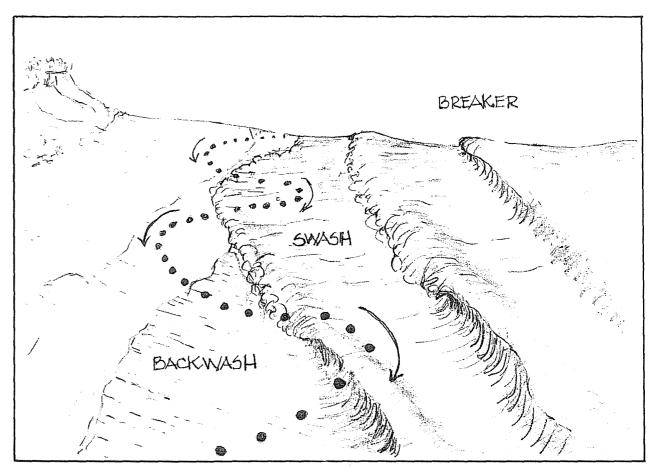
Waves striking a beach at an angle create a phenomenon known as littoral drift. In deep water a passing wave causes suspended particles to move in a circular path. But as the wave approaches the shore, this movement becomes horizontal in the direction of the wave. Suspended particles of silt or sand are then carried ashore and back out with the backwash. The dotted line indicates the general movement of sediments along the coast with the successive swash and backwash of the wave action.
