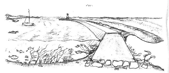
Man made structures built to stablize the shoreline often modify the environment in various ways. The pounding waves of the exposed side of the jetty above, simulate the stressful environment of the rocky shore, while the protected side may allow the estblishment of plants and animals associated with low energy ecosystems [eelgrass, tidal flats, salt marshes].
