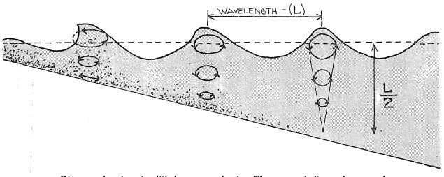
Diagram showing simplified wave mechanics. The arrows indicate the general motion of a suspended particle. The influence of a passing wave on bottom sediments is proportional to the wavelength measured crest to crest.
