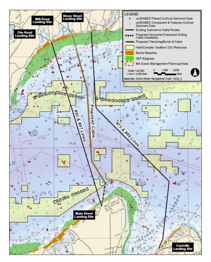
Figure 5. Proposed location of Comcast/NSTAR hybrid fiber optic/electric hybrid cable project.
