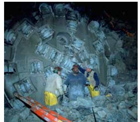
The image above was taken in 2003, just after 'hole through' near the completion of the MetroWest Tunnel. Workers are inspecting the grinding surface of the machine. At left is a diagram of the 17 mile tunnel, 200 - 500 feet below the surface.
