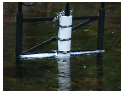
Figure 3: Hydrolab installed in frame
