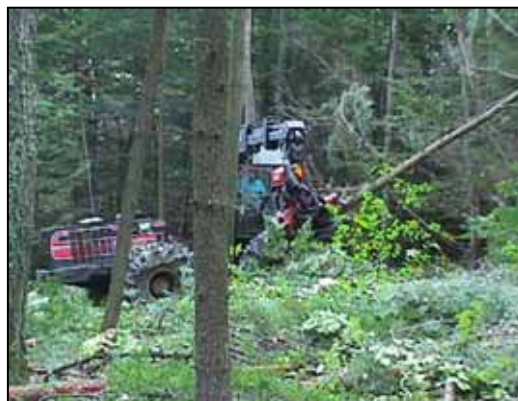
Rubber-tired C.T.L. machine with a dangle head processor
