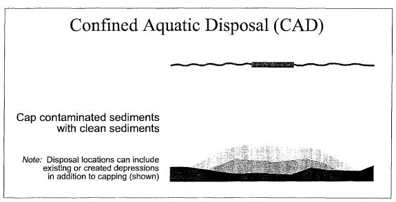
Figure 4-1: Schematic of Confined Aquatic Disposal (CAD) Method
