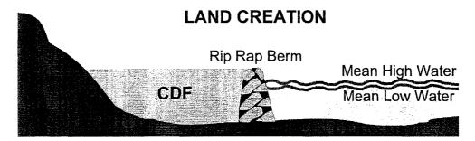
Figure 4-3: Schematic of the Confined Disposal Facility (CDF) Method
