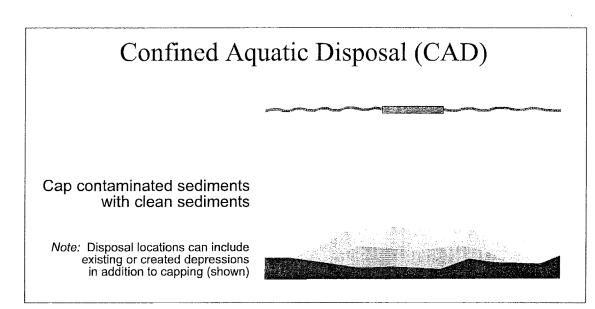
Figure 1-1: Schematic of Confined Aquatic Disposal (CAD) Method
