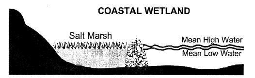
Figure 4-4: Schematic of the Tidal Habitat (TH) creation method.
