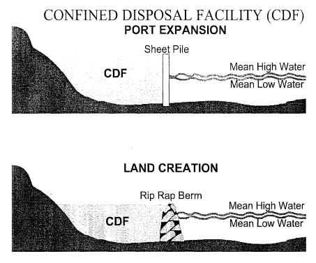
**Figure 1-3:** Schematic of the Confined Disposal Facility (CDF) Method
