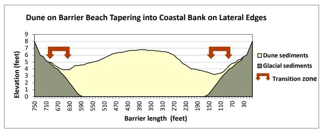
Figure 1.10. Along-shore transect showing the lateral edges of the barrier beach where the dune transitions into glacial material. The red arrows indicate the approximate location (transition zone) of the coastal bank margin of the barrier beach.
