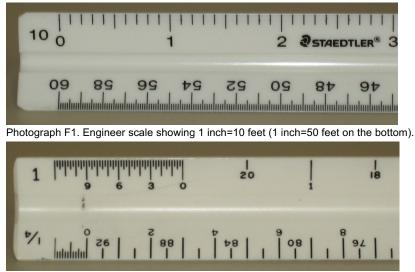
Photograph F2. Architect scale showing 1 inch=1 foot (1/4 inch=1 foot on the bottom).
