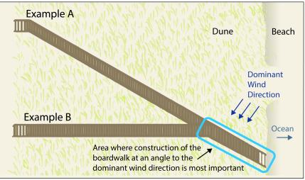
Figure 3.2. Boardwalks correctly constructed at an angle to the dominant wind direction. Example A indicates where the boardwalk would extend if it continued straight; Example B shows where the boardwalk would extend if it cut to the left and created a shorter overall distance (the break still being setback far enough from the wind).
