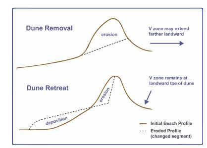
Figure 1.17. Two examples of eroded dune profiles: complete removal and retreat. The velocity zone may extend farther landward when the dune is removed. Figure modified from *Coastal Construction Manual*, FEMA.
