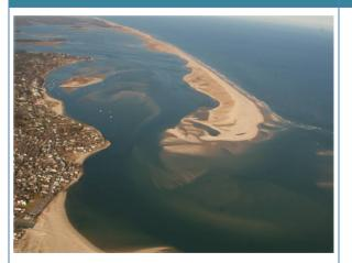
Photograph 2.10. Barrier beach with no constraint to landward movement. The barrier beach is able to shift landward since there are few alterations, developments, or constraints that would inhibit this movement.
