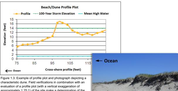
evaluation of a profile plot (with a vertical exaggeration of approximately 1.25:1) of the site make a determination of the seaward and landward boundaries of the dune easier and more accurate.
