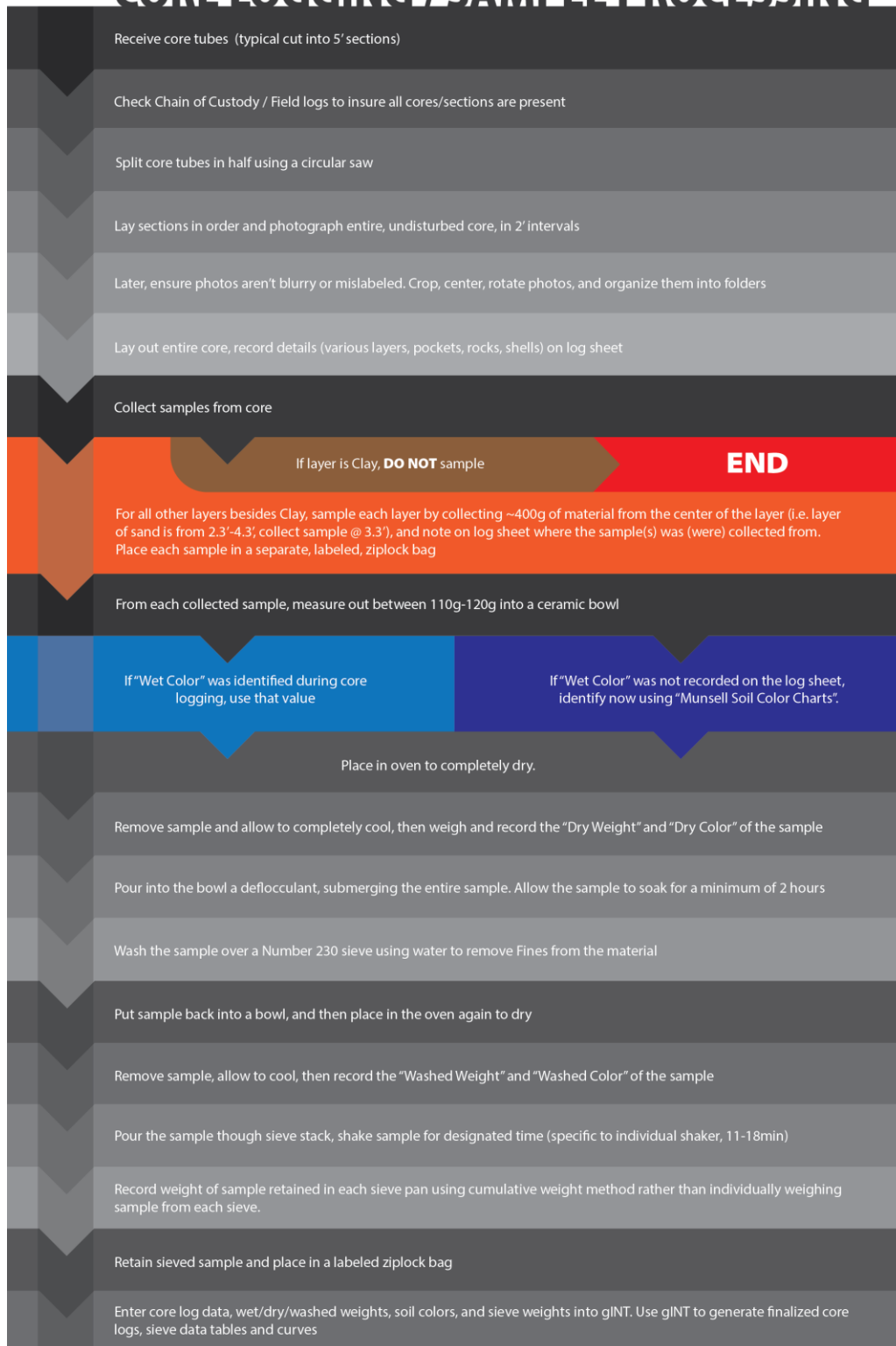
Figure 29: Flow chart depicting the steps for vibracore logging, sampling, and sample analysis.
